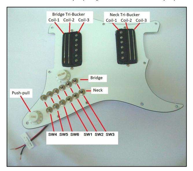
There are two "rows" of switches: The **Bridge** row and the **Neck** Row. Each row of switches controls the three pickup coils of either the Bridge TriBucker pickup or the Neck TriBucker pickup. The operation is identical for each row. For easy identification, switches now have colored covers: White for pickup coil switches, Black for parallel-series switches.
