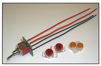
Our **Middle Pickup Switch M1** is a *user-installed* switch designed for our T4-Switch product. It gives customers with HSH pickup configuration (where two 4-wire humbucker pickups are used) added control of the middle single-coil pickup. It uses a high quality DPDT (On-Off-On) switch rated at **40,000 cycles mechanical life** for extended use without premature failure.
