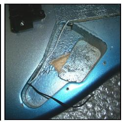
Using a hammer and wood chisel, carefully remove the identified area. These pictures show the body cavity wood being removed.
